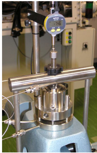
Laboratory set-up of the water uptake cell used for the study of the water uptake, swelling, and \text{NaNO}_3 leaching of non-radioactive Eurobitum samples.
