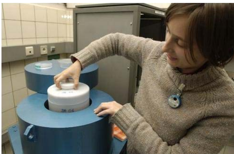
A Marinelli beaker is inserted in the lead shield containing the HPGe detector.
