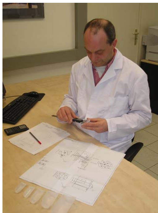
Collecting data (e.g. wall thickness) of the different vials for use in the simulation of the detector response.
