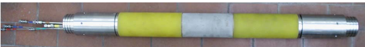
Figure 1 Adaptation of porewater pressure measurement equipment to stiff clay using packers
