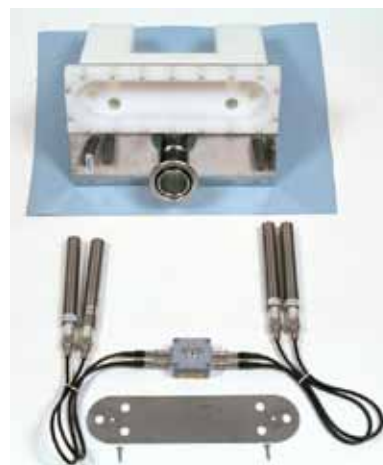
Left: Fork detector for spent fuel characterisation developed by SCK•CEN. Right: Measurements of spent fuel using the fork detector.
